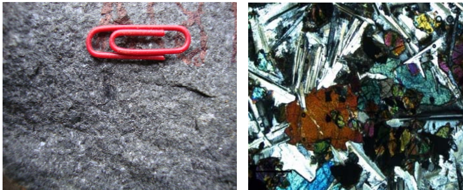
Fig.2 Left : Porphyritic pyroxene measuring up to 1cm (Paper clip = 2.8cm). Right: subophitic texture in olivine dolerite. Notice the olivine in the central parts, plagioclase laths and clinopyroxene (black bar=500 microns)
